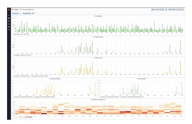
To support the One-NDS capacity expansion planning and monitoring *ndsLTA* calculates - based on the historical data and the configured RateControl-Thresholds - the date, when the system eventually reaches the engineered capacity. The calculation utilizes the average system load during the business hours and is interpolated by linear regression to the point, where it reaches the configured RateControl limits.
