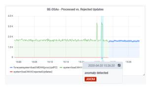
For the "Short-term Forecast" the historical data will be analyzed by STFL to forecast the next 10 minutes (blue part of the graph). In parallel to the actual incoming data deviations from the expected resp. predicted data will be checked. As soon as a significant deviation (duration and peak value) was detected, it will be marked in the chart and can be alarmed by E-Mail and/or SNMP.
