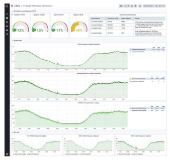
A strength of *ndsLTA* is the statistical analysis of the data. It gives the possibility to predict the system behavior for the next minutes and based on that, a detection and notification of anomalies.
